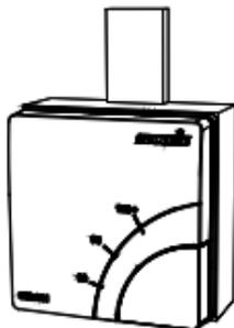
Finally switch on the mains supply and check that the SIR switches the appliance on and off correctly.
