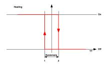
When the temperature is decreasing and reaches point 1 (defined by parameter 43), heating device is turned on and remains active until the temperature in the room is not increased to reach point 2 (defined by parameter 44). In this moment heating device is turned off.
