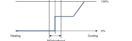
NOTE: When value is set to "0", PID inside deadband is forced to PWM minimum value. LASTVALUE means that PID remains on same level as was before entering into deadband.
